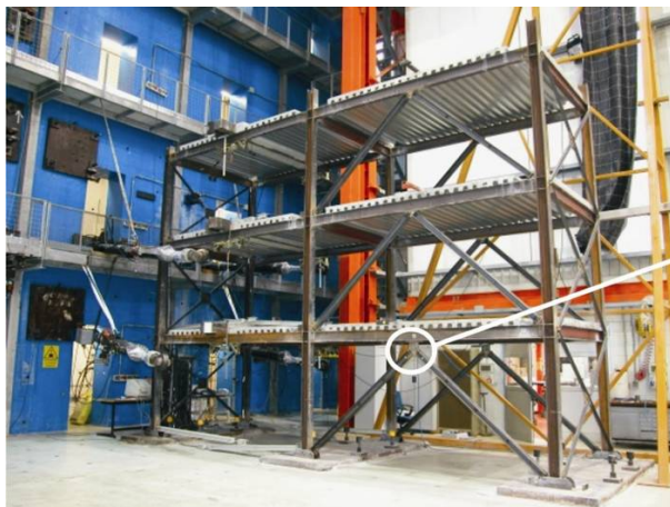
Figure 6. Half-scale steel frame at the JRC Ispra converted into a HDS by bracing the upper floors and providing a SPD as passive control device in the ground floor (white circle); and hysteresis loop of the SPD after 50 severe pseudo-dynamic earthquake simulations
