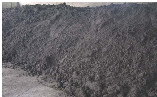
Slika 7. Sustav za pročišćavanje otpadnih voda u Zagrebu i pepeo nastao spaljivanjem mulja otpadnih voda [18] Figure 7. Water treatment plant and incinerated sewage sludge obtained as by-product [18]
